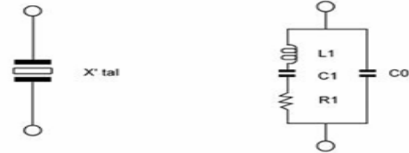
Fig 1 Equivalent Circuit of Crystal Unit
